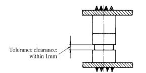
Set the tolerance clearance within 1mm to mate the male and female connectors. (Except for the lock cable type)
